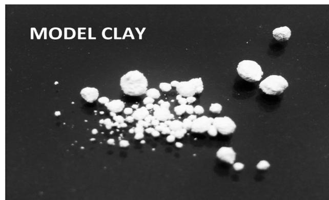
Figure 3. Kaolin (model clay) used to observe the fluorescence intensity difference between bitumen and clay.
