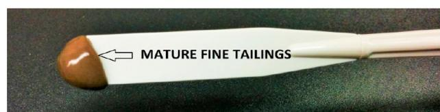
Figure 4. MFT sample from Syncrude tailings pond.
